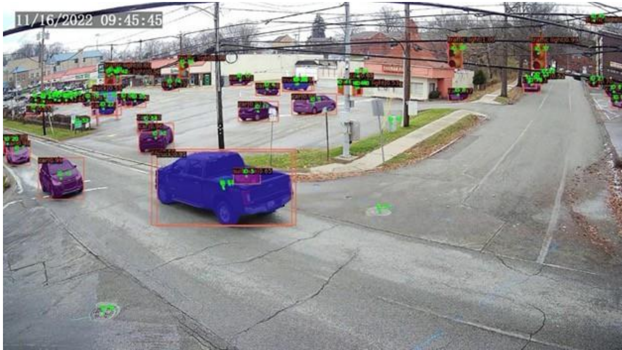
Figure 2: Example output of object detection algorithm. Detected objects are shown with a cover overlay and within a bounding box. The class name and confidence score are also shown. (Source: CMU Robotics).
